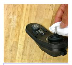
**Step 1:** Clean stem of joystick module with alcohol
